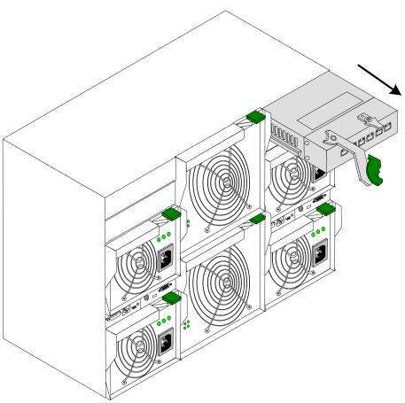
6 Place either another Ethernet Switch Module or a end-cap (blank plug) in the bay within one minute.
