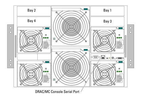
**NOTE:** To maintain proper system cooling, each module bay must contain either a module or end-cap (blank plug).
