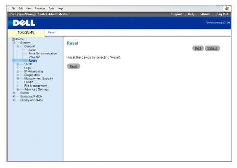
**NOTE:** Save all changes to the Startup Configuration file before resetting the switch module. This prevents the current switch module configuration from being lost. For more information about saving Configuration files, see "Managing Files" on page 158.
