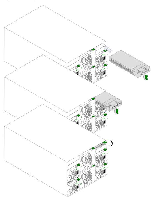
Figure 3-9. Inserting a Ethernet Switch Module into the
