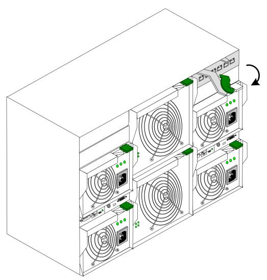
**5** Slide the Ethernet Switch Module out of the Dell Modular Server Chassis and set it aside.
